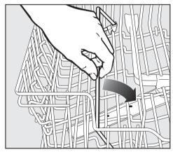
The coffee bar can be flipped over to the middle of the basket for easy sorting and unloading.
